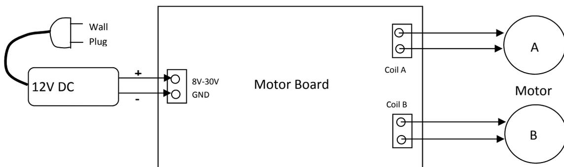
When making your connections BE SURE to get the correct polarity on the 12V DC connector. If you reverse the connection the motors will not run, and you may possibly burn something on the motor board.
