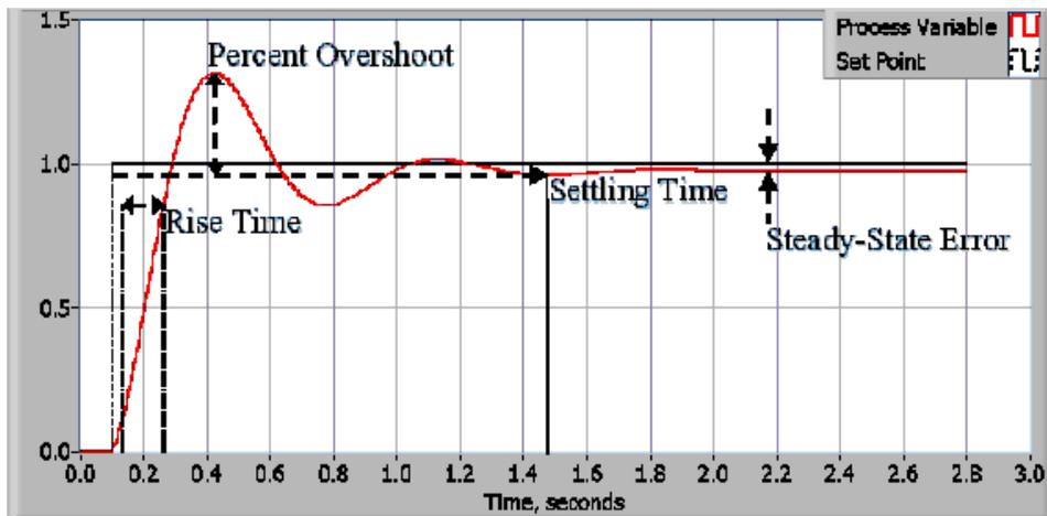
Here we would say the steady-state response is achieved in about 1.5 seconds with an initial rise time of around 150 milliseconds and a 30% initial overshoot. If objectionable, the remaining steady-state error might be “cured” by adding some integral action
